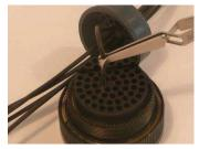
5.3.3 Using the correct insertion tool for the contact as shown above, locate onto contact bucket and push the contact forward until fully inserted, when a 'click' will be heard and felt.
