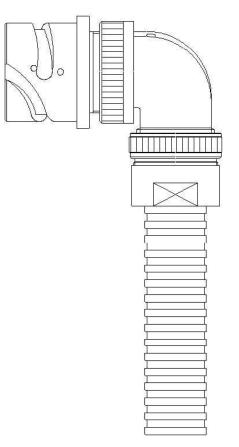
Example of finished Assembly (90°Degree Elbow)
