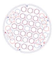
Example of two 40-A35 Contact arrangements with X and Y orientations mated together. 25 out of the 35 available contacts can misalign.
