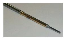
Slide the tool out and remove the tool from the wire.
