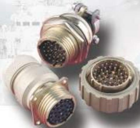
**Mk18 (Pattern 608).** A complete system of medium density connectors and accessories designed to withstand extreme environmental conditions. Meeting the requirements of BS9522-F0020, Mk18 connectors are particularly suitable for exposed areas in marine and land based equipments. The nickel aluminium bronze shells provide excellent corrosion resistance coupled with high strength.
