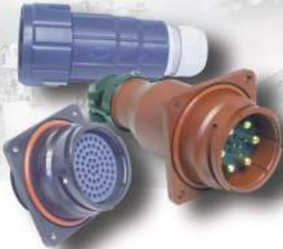
**ABCIRH Size 49.** Shell size 49 connectors are used principally in Rail Transportation for the inter-car and inter-unit jumper cable assemblies. The connectors have all the high performance features of the standard ABCIRH range. Polarisation is achieved by 5 key / keyway system and the free plug is supplied with a rubber covered coupling nut designed to withstand flying ballast and possible damage caused by being accidentally dropped onto a hard surface.
