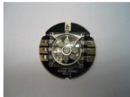
Test set-up on MCPCB
