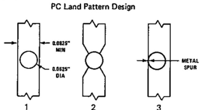
The two desirable factors are: To have as much surface area of land pattern adjacent to the unit as possible to ensure support of both lens mounting tabs to prevent tilting, and to provide mechanical strength of land pattern when unit is being reworked or removed.
