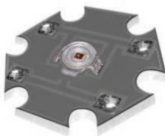
*LEDs on Anotherm<sup>®</sup> substrates provide the necessary heat dissipation requirements*
