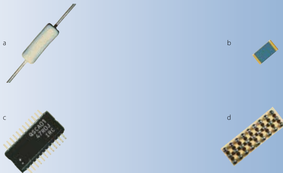
Fig.2. Tested terminators. (a) Axial leaded resistor. (b) 0603 chip. (c) QSOP. (d) BGA.
